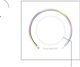
Click the knob to switch ON/OFF. Press and hold down to adjust brightness to 100%. Double click the knob to switch between RGB color mode and brightness mode.
