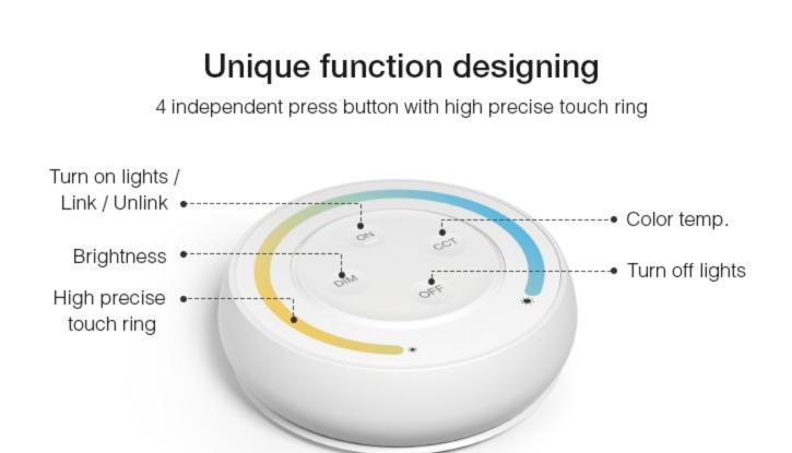
Right and left sliding touch ring for dimming brightness / color temp.
