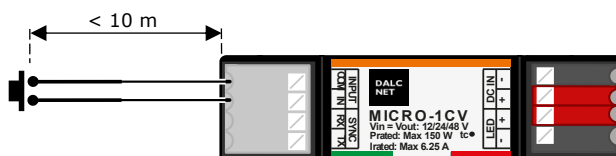
Figure 3: Push-button wiring diagram recommended for Short Distances
