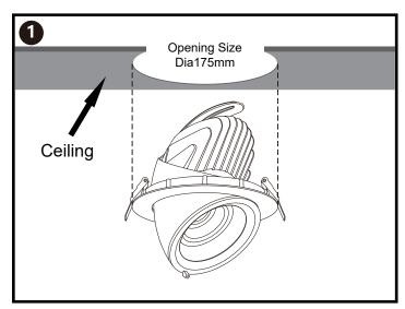
Prepare everything needed for installtion & drill a hole with diameter 175mm in the ceiling.
